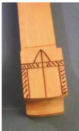
► Pic.18 The heel and wedge slots marked out
